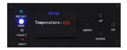
3. X-axis direction: MENU-- X Reverse Setup-- OK -- UP/DOWN
