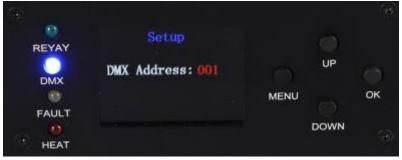
2. Temperature adjustment: MENU-- Temperature Setup --OK -- UP/DOWN (Temperature range: 580-650 degree, presetting: 620 degree)
