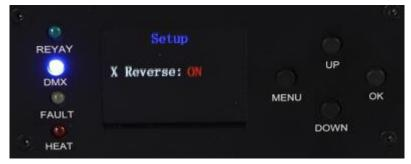
4. Y-axis direction: MENU -- Y Reverse Setup -- OK -- UP/DOWN
